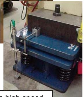
Installation of a high-speed press on VSVL2408 Isolators
